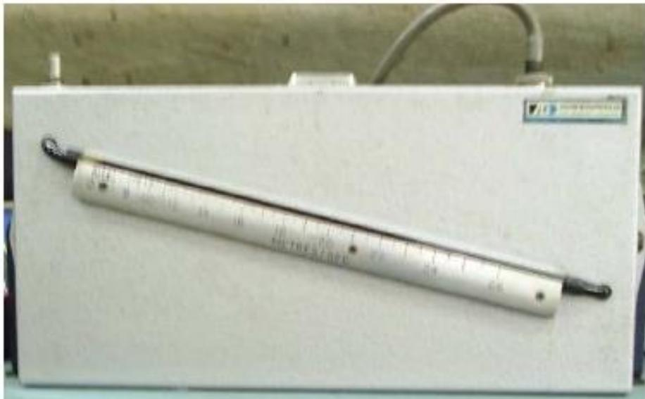
Gambar 5.5. Manometer Miring
