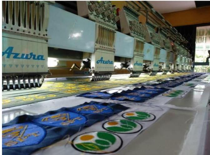
Gambar 1.1 Mesin bordir computer
