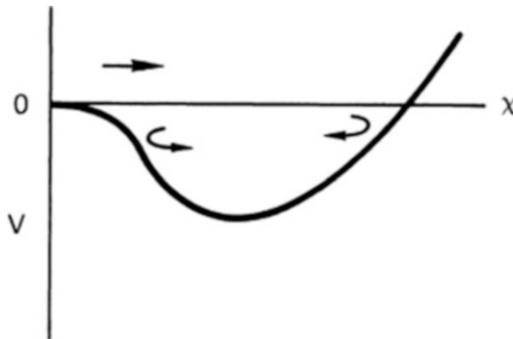
**Fig. 8.6** The Sagdeev potential  $V(\chi)$ . The *upper arrow* is the trajectory of a quasiparticle describing a soliton: it is reflected at the right and returns. The *lower arrows* show the motion of a quasiparticle that has lost energy and is trapped in the potential well. The bouncing back and forth describes the oscillations behind a shock front
