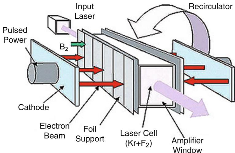
**Fig. 10.65** Diagram of a krypton-fluoride laser amplifier [J.D. Sethian et al., *Phys. Plasmas* **10**, 2142 (2003)]
