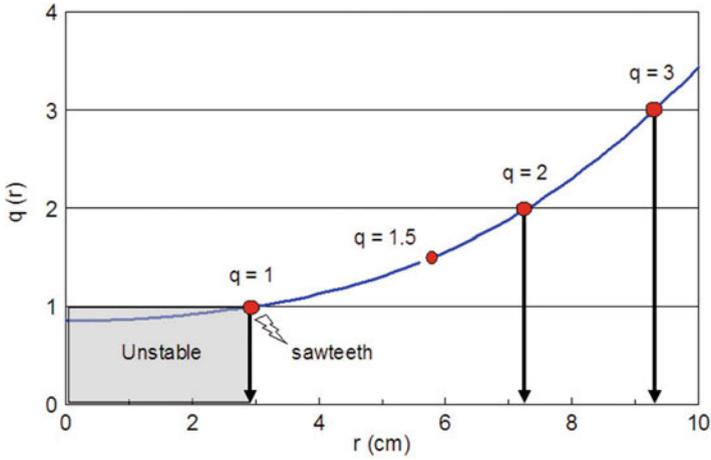
Fig. 10.28 A typical  $q$  profile in a tokamak
