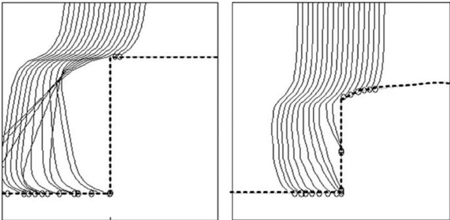
**Fig. 10.75** Deflections of the orbits of ions from the plasma at the top caused by surface charges on the mask, for a square trench entrance (*left*), and a rounded one (*right*) [T.G. Madziwanussinov, D. Arnush, and F.F. Chen, *Phys. Plasmas* **15**, 013503 (2008)]
