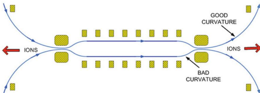
Fig. 10.16 Formation of an ion beam outside a simple mirror
