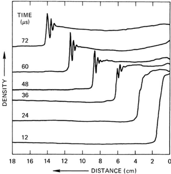
Fig. 8.11 Measurements of the density distribution in a shock wave at various times, showing how the characteristic shape of Fig. 8.5 develops. [From Taylor *et al.*, *loc cit.*]
