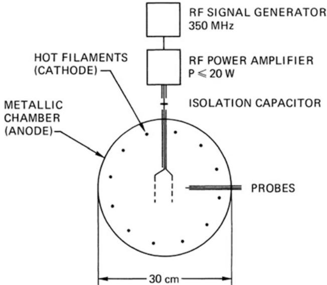
**Fig. 8.16** Schematic of an experiment in which the parametric decay instability was verified. [From A. Y. Wong *et al.*, *Plasma Physics and Controlled Nuclear Fusion Research*, 1971, I, 335 (International Atomic Energy Agency, Vienna, 1971).]
