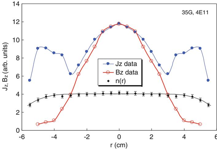
**Fig. 9.13** Radial profiles of  $n(r)$ ,  $B_z(r)$ , and  $J_z(r)$  in a helicon discharge at  $B=3.5$  mT and  $n=4 \times 10^{17} \text{ m}^{-3}$  (D.D. Blackwell, T.G. Madziwa, D. Arnush, and F.F. Chen, *Phys. Rev. Lett.* **88**, 145002 (2002))
