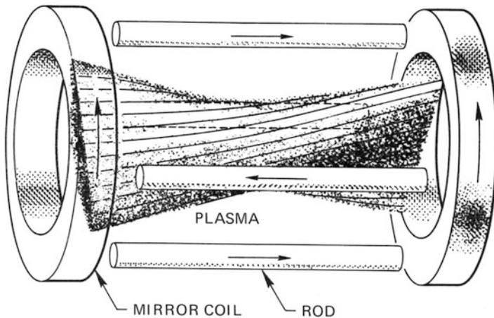
**Fig. 10.12** A magnetic mirror with Ioffe bars
