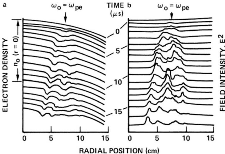
**Fig. 8.30** Coupled electron and ion wave solitons. In (a) the low-frequency density cavities are seen to propagate to the left. In (b) the high-frequency electric field, as measured by wire probes, is found to be large at the local density minima. [From H. Ikezi, K. Nishikawa, H. Hojo, and K. Mima, *Plasma Physics and Controlled Nuclear Fusion Research*, 1974, II, 609, International Atomic Energy Agency, Vienna, 1975.]
