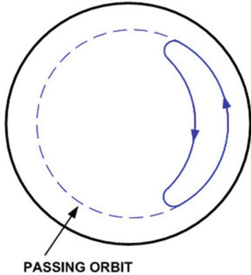
**Fig. 10.34** Mechanism of the Ware Pinch
