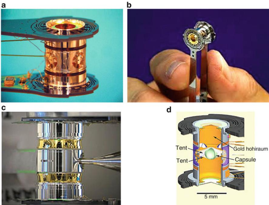
**Fig. 10.59** Hohlraums: (a) a hohlraum in its holder; (b) size of a hohlraum; (c) a “rugby” hohlraum with an ellipsoidal cavity; (d) suspension of a capsule in a hohlraum with thin plastic membranes or “tents”
