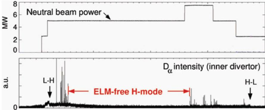
Fig. 10.37 An ELM-free discharge in ASDEX-U [Suttrop et al., Plasma Phys. Control. Fusion 45, 1399 (2003)]
