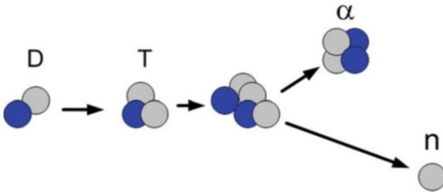
**Fig. 10.2** Diagram of the D–T reaction
