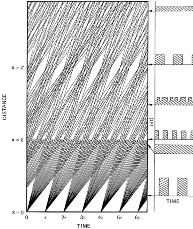
**Fig. 8.20** Space-time trajectories of gated particles showing the bunching that causes echoes. The density at various distances is shown at the right. [From D. R. Baker, N. R. Ahern, and A. Y. Wong, *Phys. Rev. Lett.* **20**, 318 (1968).]
