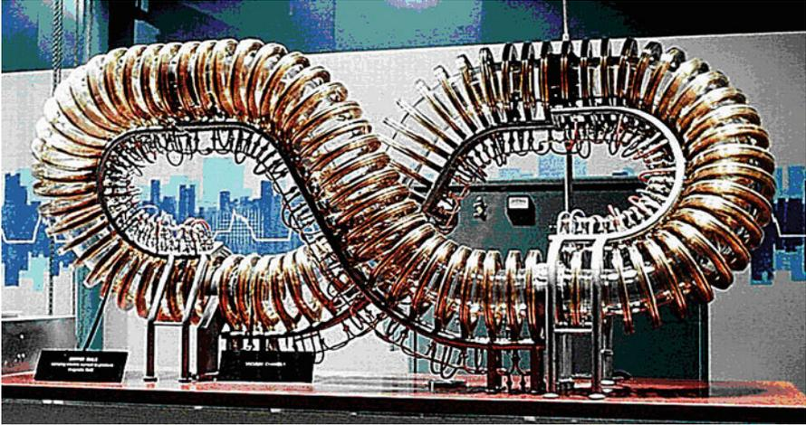
**Fig. 10.23** Exhibit model of a figure-8 stellarator
