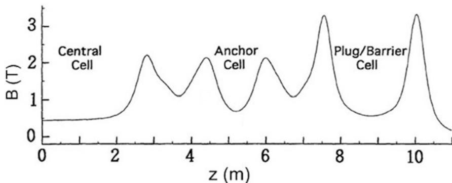
Fig. 10.15 Magnetic field configuration in a tandem mirror
