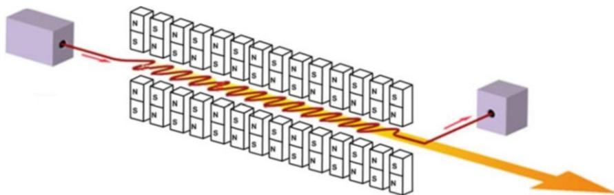
Fig. 10.56 Diagram of a free-electron laser (FEL)
