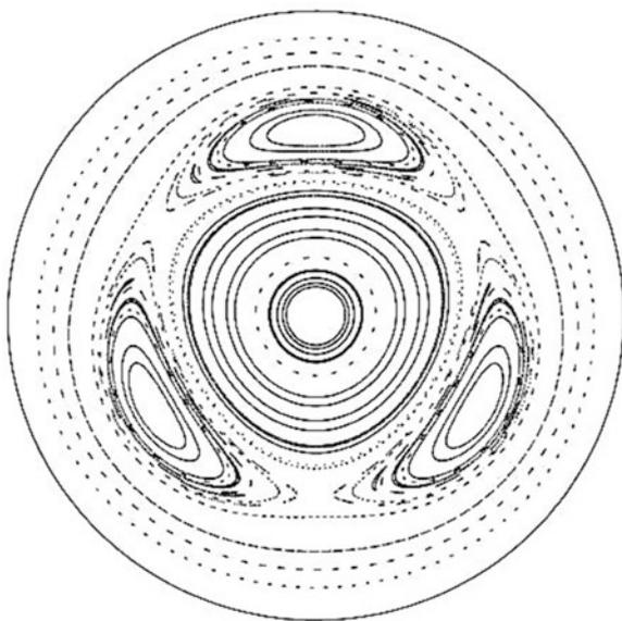
**Fig. 10.32** Mirror-trapping of a particle in a torus
