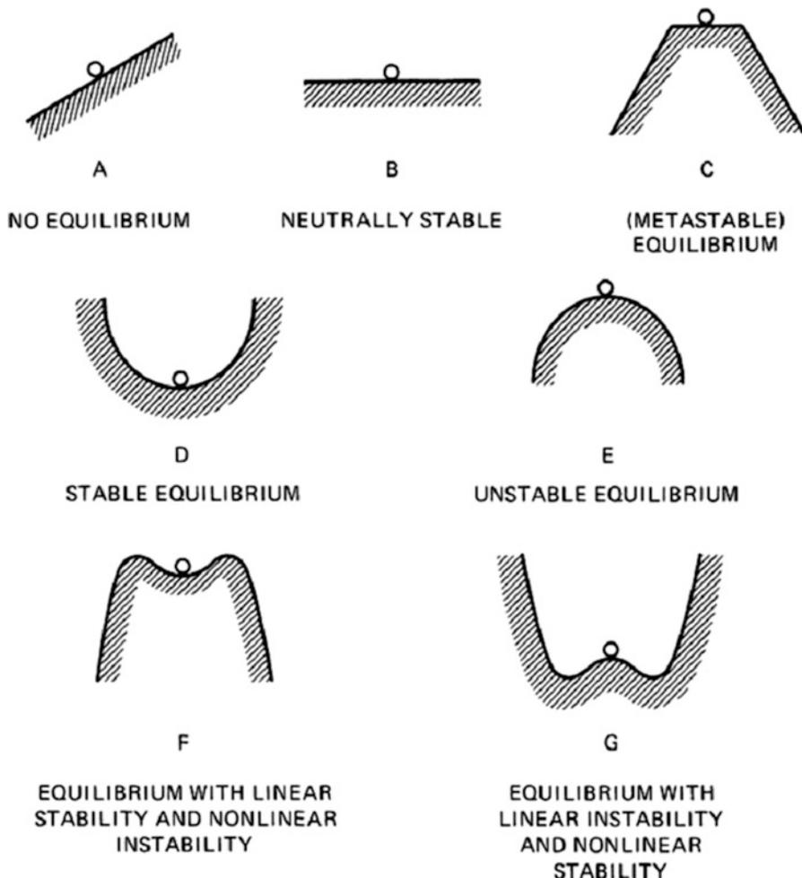
Fig. 6.1 Mechanical analogy of various types of equilibrium
