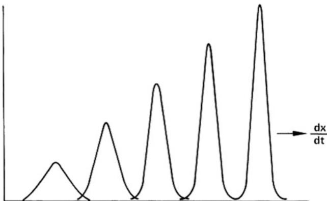
**Fig. 8.25** A train of solitons, generated at the *left*, arrayed according to the relation among speed, height, and width
