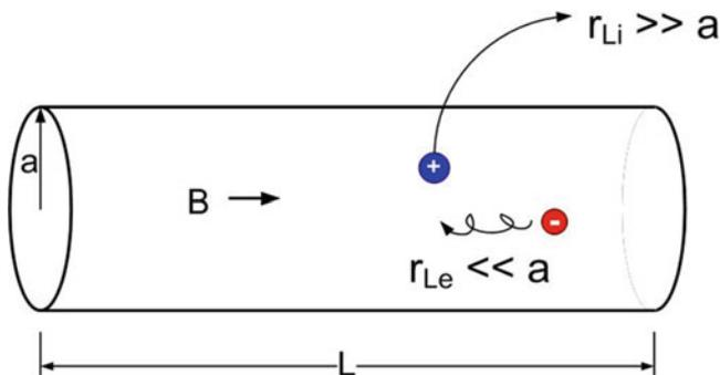
Fig. 8.43 Model of a finite-length laboratory plasma
