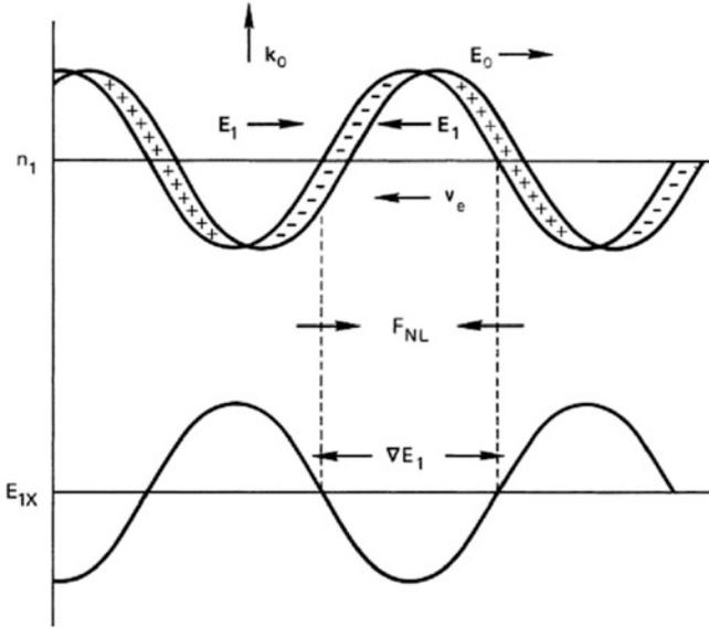
Fig. 8.15 Physical mechanism of the oscillating two-stream instability
