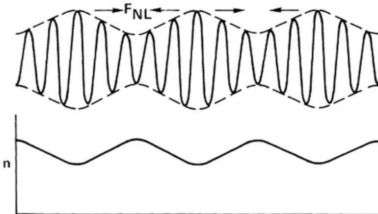
**Fig. 8.26** The ponderomotive force of a plasma wave with nonuniform intensity causes ions to flow toward the intensity minima. The resulting density ripple traps waves in its troughs, thus enhancing the modulation of the envelope
