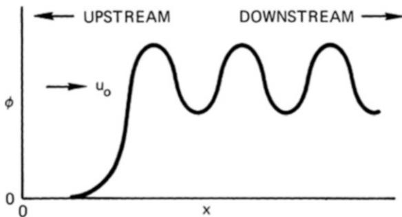
$$\chi \equiv + \frac{e\phi}{KT_e} \quad \xi \equiv \frac{x}{\lambda_D} \quad \mathcal{M} \equiv \frac{u_0}{(KT_e/M)^{1/2}} \quad (8.26)$$
