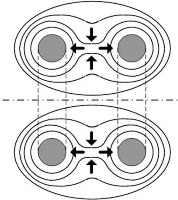
field lines move in the direction of the arrows, and a reconnection sheet of horizontal cross section forms. If the current is increased, the field lines move opposite to the arrows, and the reconnection sheet has a vertical cross section.
