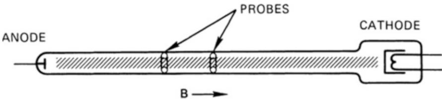
**Fig. 5.14** The Lehnert-Hoh experiment to check the effect of a magnetic field on diffusion in a weakly ionized gas
