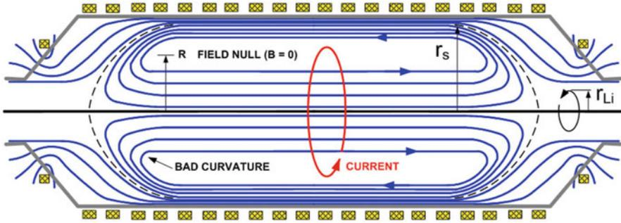
**Fig. 10.18** Geometry of an RFX. The dashed line is the separatrix, with maximum radius  $r_s$
