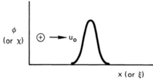
well ( $x > 0$ ), reflect, and return to  $x = 0$ , making a single transit. Similarly, a quasiparticle in our analogy will make a single excursion to positive  $\chi$  and return to  $\chi = 0$ , as shown in Fig. 8.7. Such a pulse is called a *soliton*; it is a potential and density disturbance propagating to the left in Fig. 8.7 with velocity  $u_0$ .
