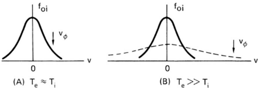
**Fig. 7.30** Explanation of Landau damping of ion acoustic waves. For  $T_e \approx T_i$ , the phase velocity lies well within the ion distribution; for  $T_e \gg T_i$ , there are very few ions at the phase velocity. Addition of a light ion species (*dashed curve*) increases Landau damping
