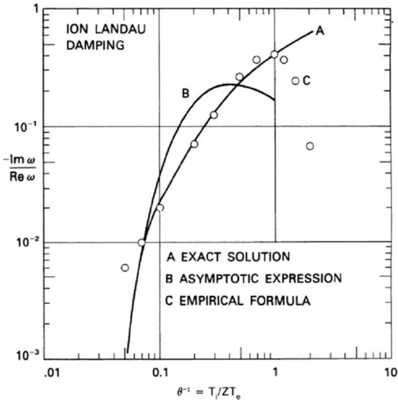
**Fig. 7.31** Ion Landau damping of acoustic waves. (A) is the exact solution of Eq. (7.128); (B) is the asymptotic formula, Eq. (7.133); and (C) is the empirical fit, Eq. (7.134), good for  $1 < \theta < 10$ .
