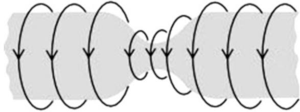
**Fig. 10.6** Mechanism of a kink instability
