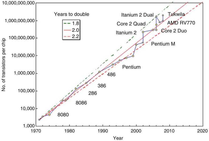
Fig. 10.66 Moore's law of transistors on a chip
