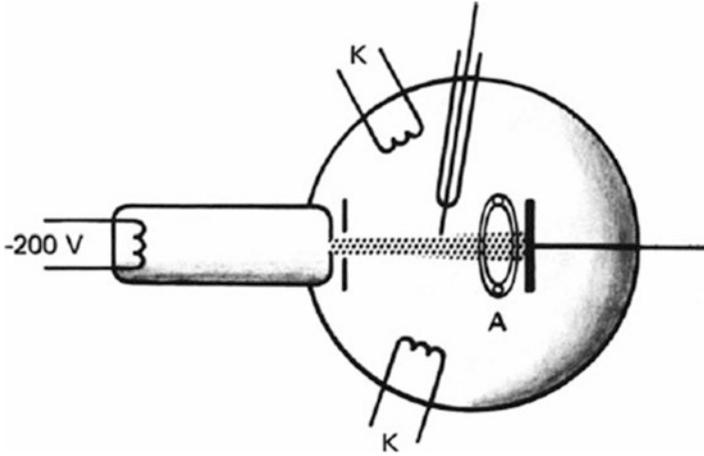
**Fig. 4.6** Schematic of the Looney–Brown experiment on plasma oscillations
