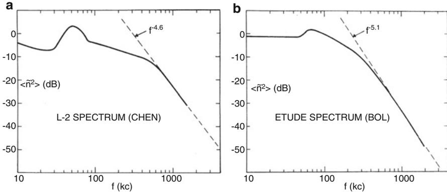
**Fig. 8.38** Turbulence spectra in (a) the L-2, a reflex arc ( $2000\text{ G}$ ,  $10^{12}\text{ cm}^{-3}$ ); and (b) the Etude, a stellarator ( $6700\text{ G}$ ,  $10^{13}\text{ cm}^{-3}$ ). Here, frequency is measured rather than  $k$
