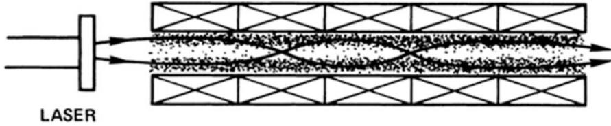
**Fig. 4.31** A plasma confined in a long, linear solenoid will trap the CO<sub>2</sub> laser light used to heat it only if the plasma has a density minimum on axis. The vacuum chamber has been omitted for clarity
