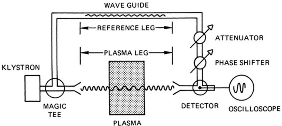
Fig. 4.28 A microwave interferometer for plasma density measurement
