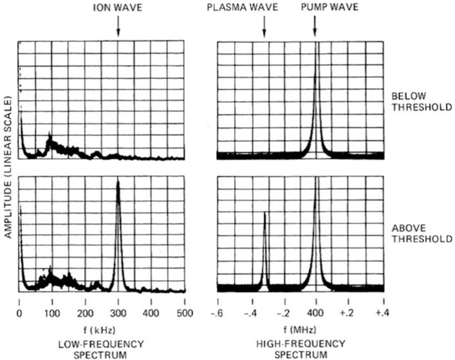
**Fig. 8.17** Oscilloscopes showing the frequency spectra of oscillations observed in the device of Fig. 8.16. When the driving power is just below threshold, only noise is seen in the low-frequency spectrum and only the driver (pump) signal in the high-frequency spectrum. A slight increase in power brings the system above threshold, and the frequencies of a plasma wave and an ion wave simultaneously appear. [Courtesy of R. Stenzel, UCLA.]
