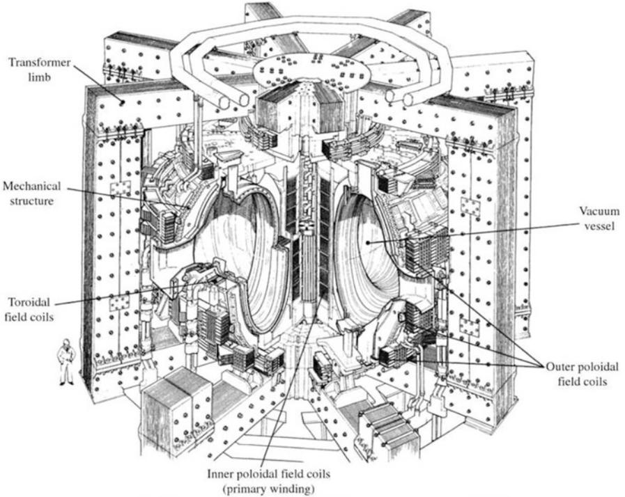
**Fig. 10.40** Diagram of the JET tokamak in the U.K. [J. Wesson, *Tokamaks*, Oxford Science Publications (1987), p 658]
