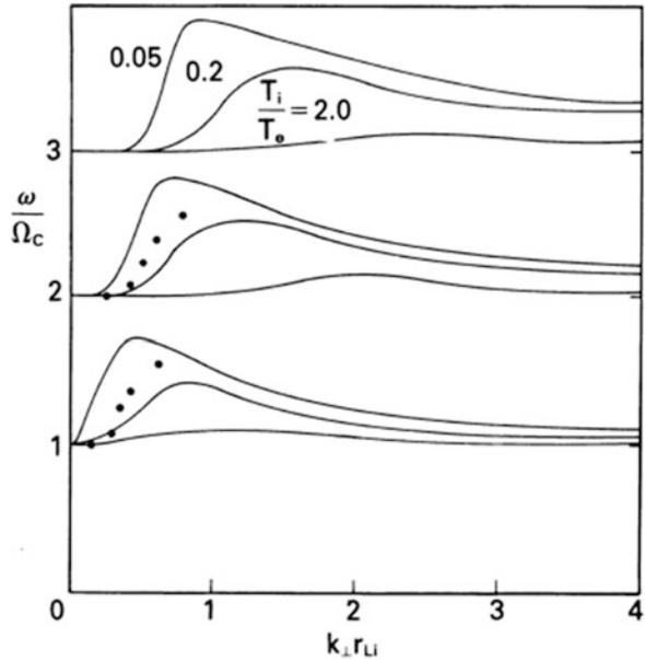
Eq. (7.160) must be large; and this can happen only near a resonance  $\omega \simeq n\Omega_c$ . Thus the neutralized modes are not sensitive to the lower hybrid resonance  $\omega \simeq \omega_l$ . Indeed, as  $k_{\perp} r_{Li} \rightarrow 0$  the envelope of the dispersion curves approaches the electrostatic ion cyclotron wave relation (4.67), which is the fluid limit for neutralized waves.
