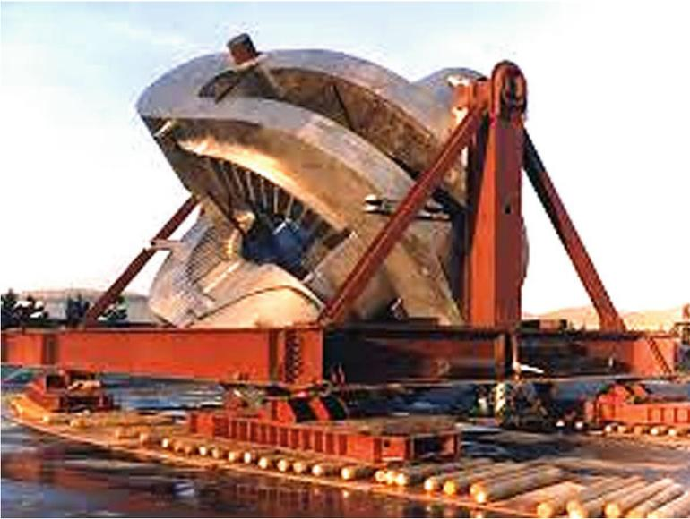
**Fig. 10.14** The MFTF-B mirror machine being moved by the old Roman method
