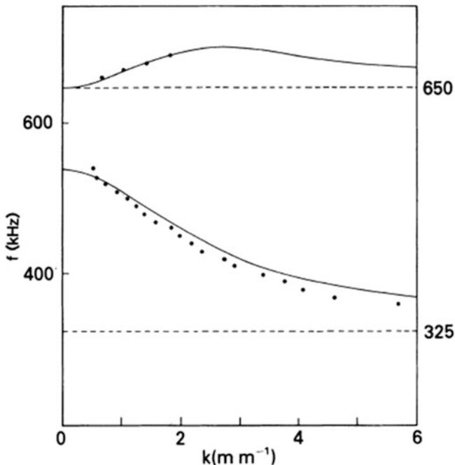
**Fig. 7.35** Pure ion Bernstein waves: agreement between theory and experiment in a  $Q$ -machine plasma [From J. P. M. Schmitt, *Phys. Rev. Lett.* **31**, 982 (1973)]
