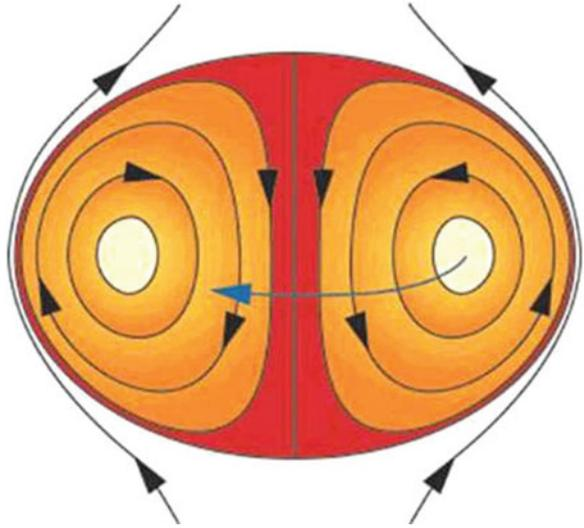
A diagram of a spheromak is shown in Fig. 10.48. A toroidal current creates an entirely poloidal B-field, and there is no central core. This is formed by injecting a plasma with the right helicity into a flux conserver, as shown in Fig. 10.49.
