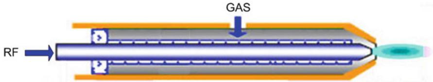
Fig. 9.17 Schematic of a pencil-type atmospheric plasma
