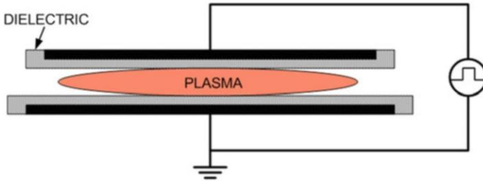
**Fig. 9.15** A dielectric barrier discharge of Type 1
