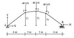
Fig. E6.9c Optimal shape
