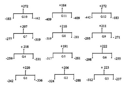
Fig. 15.22 Maximum and minimum design moments (kip ft)
