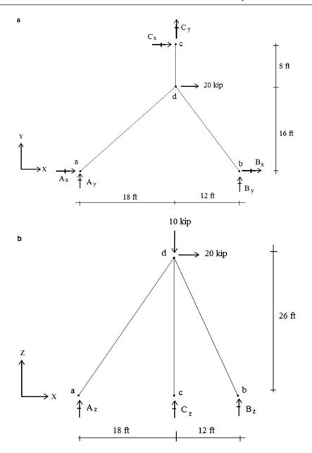
**Fig. E2.26** Tripod geometry and supports. (a) x - y plan view. (b) x - z plan view
