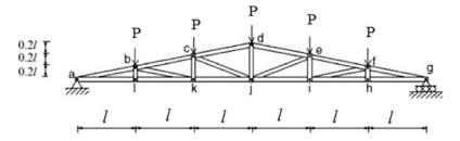
Fig. E2.17a Geometry and loading
