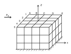
**Fig. 14.24** Shear model of typical frame
