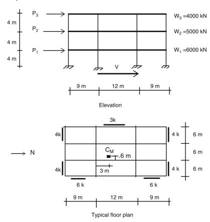
**Problem 14.4** Consider the two-story rigid frame defined below. Assume the weight of the floor slabs is equal to  $w_{\text{floor}}$ . Concentrated masses are located on each floor as indicated.
