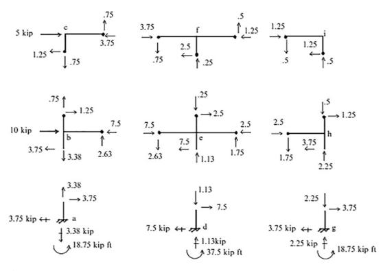
Fig. E11.2g Axial and shear forces (kip)
