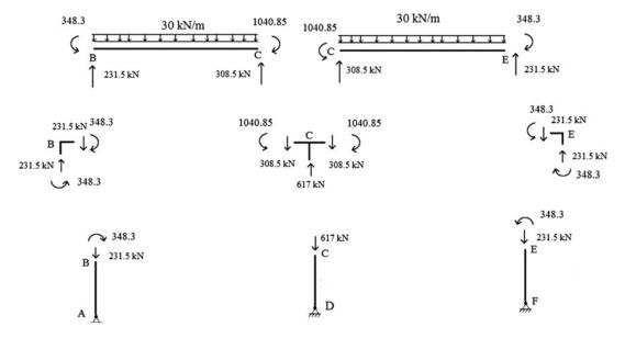
Fig. E10.14d Free body diagram
