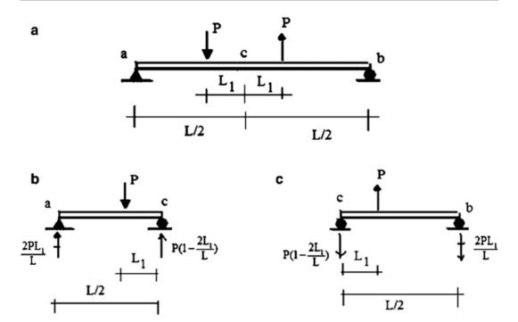
Fig. 3.49 Bending conditions on symmetry axis—anti-symmetrical planar loading. (a) Anti-symmetrical planar load. (b) Left segment. (c) Right segment
