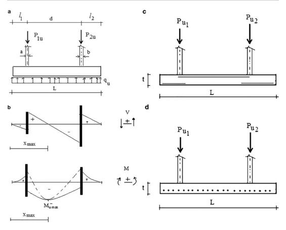
**Fig. 7.15** (a) Rectangular footing with uniform ultimate soil pressure  $e_{\rm u}=0$ . (b) Shear and Moment diagrams  $e_{\rm u}=0$ . (c) Steel reinforcing pattern for longitudinal bending. (d) Steel reinforcing pattern for transverse bending
