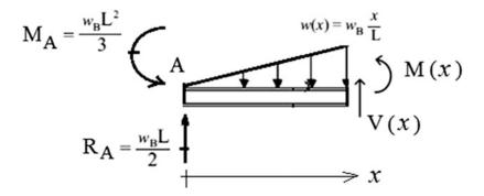
Fig. E3.10c Internal shear and moment
