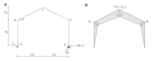
**Fig. 9.53** (a) Primary structure-unit load. (b)Bending moment distribution for  $H_E = 1$
