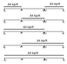
arbitrary value for *I* since the moment results are independent of *I*. Computer-based analysis is ideally suited for envelopes. Certain software packages have incorporated special features that automate the process of moving the load across the span and compiling the peak positive and negative moment values at each discrete section. Both the positive and negative moment envelopes are required in order to dimension the beam cross section.
