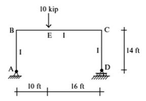
**Problem 4.38** Determine the horizontal deflection at C.  $I = 100(10)^6 \text{ mm}^4$  and E = 200 GPa. Sketch the deflected shape. Use the Virtual Force method.
