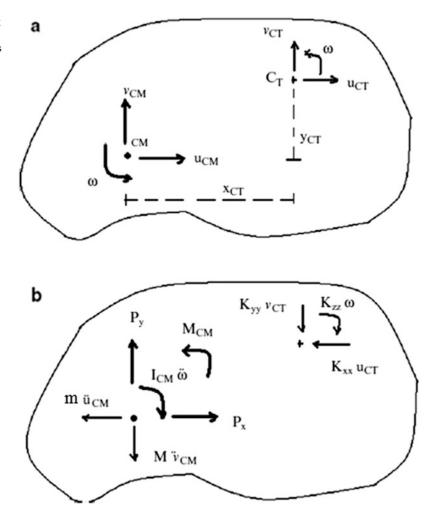
When the loading is dynamic, one needs to include the inertia forces. In this case, it is more convenient to place the origin at the center of mass and work with force and displacement quantities referred to the axes centered at the center of mass. Figure 14.18a illustrates this choice. Note that the resistance forces act at the center of twist and produce a moment about the center of mass. The displacements of the two centers are related by
