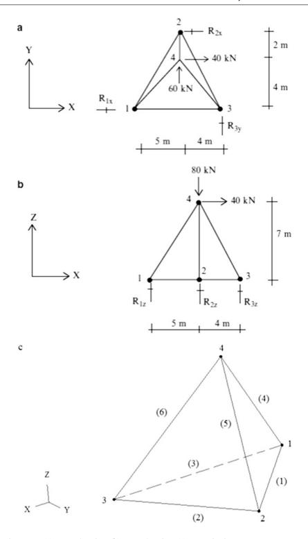
**Fig. E2.28** 3-D Truss. (a) x - y plan view. (b) x - z plan view. (c) Isometric view
