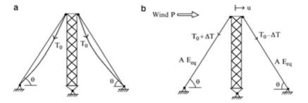
We develop an expression for  $E_{eq}$  by modifying (5.25). Figure 5.23 shows a typical inclined cable and the notation introduced here. The loading acting on the cable is assumed to be the self weight, wg. Also when the cable is rotated from the horizontal position up to the inclined position, H is now the cable tension, T; the normal distributed load w becomes  $w_g \cos \theta$ ; and the loading term becomes
