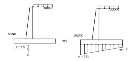
Example 8.5 Retaining Wall Supported by Concrete Piles
