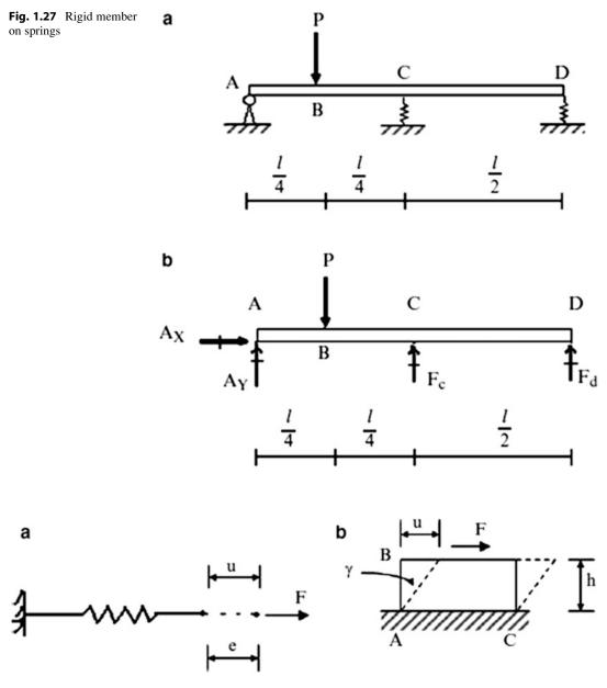
Fig. 1.28 Deformation modes. (a) Extension. (b) Shear
