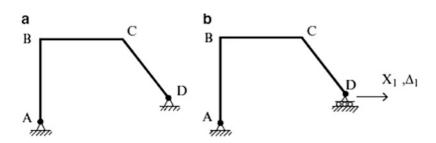
**Fig. 9.32** (a) Actual structure. (b) Primary structure—redundant reactions
