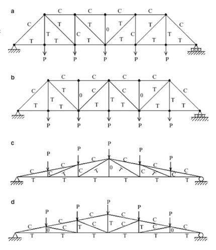
As an example, consider the two diagonal patterns shown in Fig. 2.29a, b. The sense of the member forces due to a uniform live load is indicated by C (compression) and T (tension).
