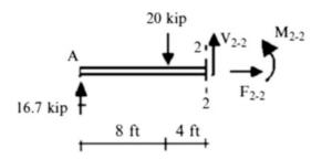
**Fig. E1.3d** Left segment-cutting plane 2-2
