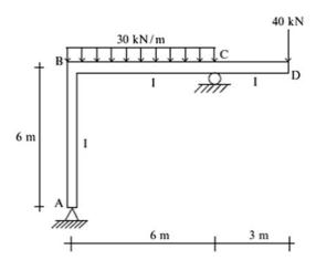
**Problem 4.34** Determine the horizontal displacement at joint B. Take E = 29,000 ksi and I = 200 in. Use the Virtual Force method.
