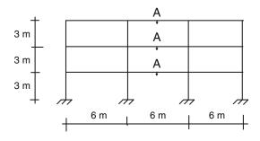
Using Müller-Breslau Principle, determine the loading patterns (uniformly distributed member load) that produce the peak values of positive moment at point A (mid-span) for each story.
