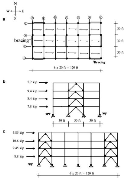
The braces have equal stiffnesses and the floors are rigid. Therefore the global wind load will be distributed equally between braces (see Chap. 14). The column load is purely axial since the members are pinned. We establish the column load per floor working with the tributary floor area associated with the column. The beams are simply supported, and the beam loading is based on one-way action (uniformly loaded).
