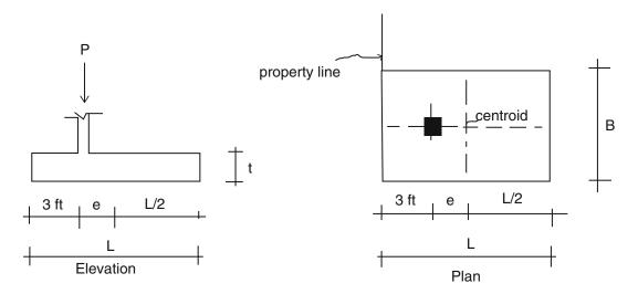
Fig. E7.2c Geometry and loading
