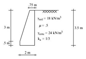
**Problem 8.2** For the concrete retaining wall shown, determine the factors of safety against sliding and overturning and the base pressure distribution. Use the Rankine theory for soil pressure computations.
