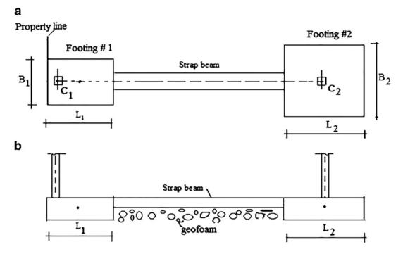
Fig. 7.16 Strap footing. (a) Plan. (b) Elevation
