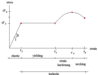
**Fig. 16.2** Steel properties—structural steels
