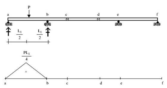
Fig. E3.27b Moment diagram—load on member AB
