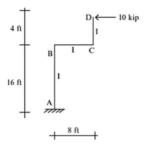
**Problem 4.33** Determine the vertical deflection at D and the rotation at joint B. Take E = 200 GPa and  $I = 60(10)^6$  mm<sup>4</sup>. Use the Virtual Force method.
