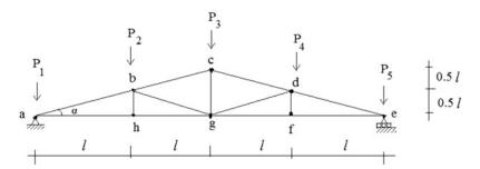
Fig. E2.20a Structural geometry and nodal loads
