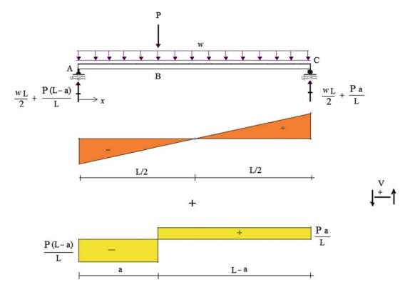
Fig. E3.11c Shear diagrams
