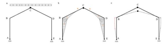
Fig. 4.30 3-Hinge gable frame. (a) Loading. (b) Bending moment. (c) Deflection profile
