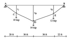
Fig. E5.1a Cable geometry and loading
