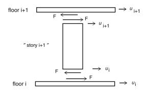
**Fig. 14.20** Forces acting on floor i
