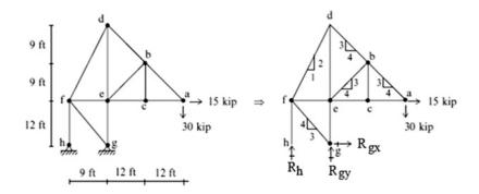
Fig. E2.7a Solution: First, we determine the zero force members. Starting at joint c, we observe that  $F_{\rm cb}=0$ . Then, moving to joint b, it follows that  $F_{\rm be}=0$ .
