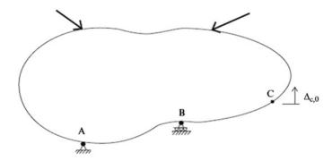
**Fig. 9.4** Displacement due to unit value of  $R_{\rm C}$
