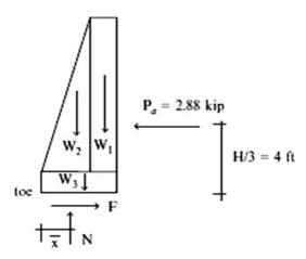
Fig. E8.1b Free body diagram
