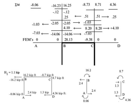
Fig. E10.17c Case I-end moments and column shear
