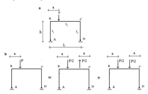
Fig. 9.40 (a) Two-hinged frame under gravity loading. (b) Decomposition of loading into symmetrical and antisymmetrical components
