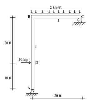
**Problem 4.31** Determine the value of I to limit the vertical deflection at C to 30 mm. Take E = 200 GPa. Use the Virtual Force method.
