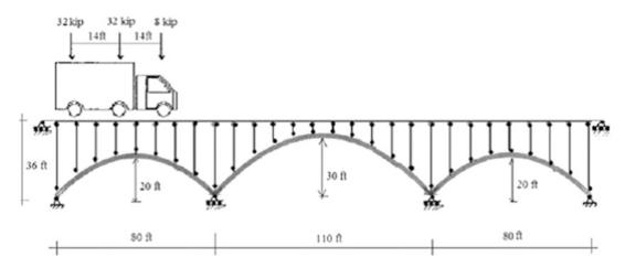
Fig. 13.31 Idealized model—three-span arch
