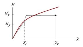
Fig. 16.8 Moment–curvature relationship—concrete beams
