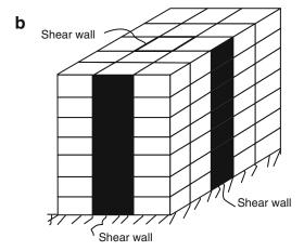
Fig. 14.2 (a) Steel braced frame with bracing. (b) Concrete frame with shear walls
