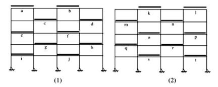
Fig. E15.1b Positive moment loading patterns
