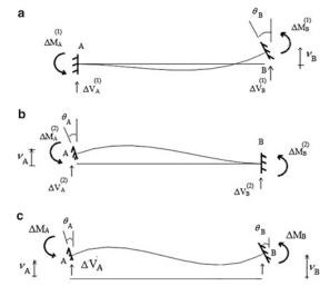
**Fig. 10.9** (a) Support A fixed. (b) Support B fixed
