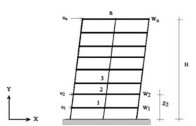
where u(H) is the relative displacement of the top floor with respect to the ground, and  $Z_i$  is the vertical coordinate of floor i. This assumption leads to the following expression for the total acceleration of a typical floor:
