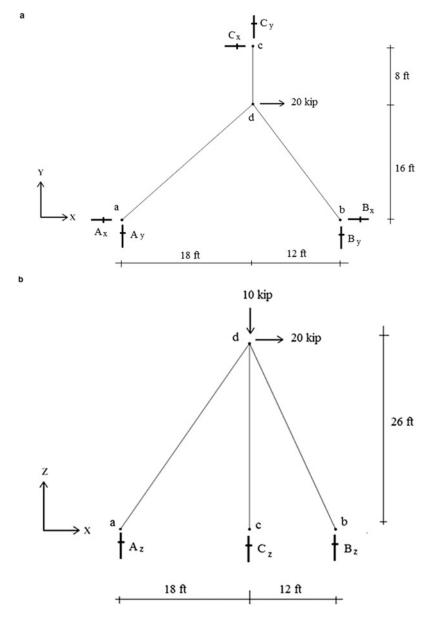
**Fig. E2.24** Tripod geometry and supports. (a) x - y plan view. (b) x - z plan view
