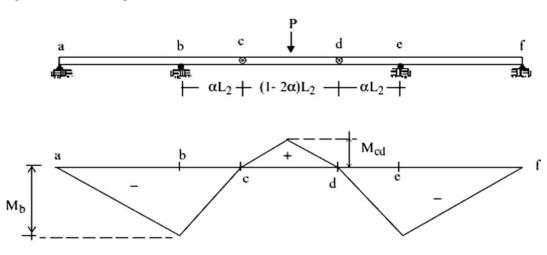
**Fig. E3.27d** Moment diagram—load on member CD Based on these analyses, the design moments for the individual spans are
