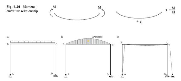
Fig. 4.27 Portal frame. (a) Loading. (b) Bending moment. (c) Deflection profile
