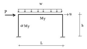
**Problem 16.6** Using computer software, generate the plot of  $u_A$  vs. P, and estimate  $P_{\text{max}}$ . Take w=1.5 kip/ft, h=12 ft, and L=30 ft. The material is steel,  $\sigma_y=50$  ksi. The exterior columns are W16  $\times$  89, the interior columns are aW16  $\times$  100, and all the beams are W24  $\times$  131.
