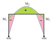
Fig. E9.15c Bending moment distribution
