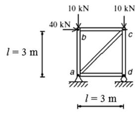
Fig. E2.13a Geometry and loading
