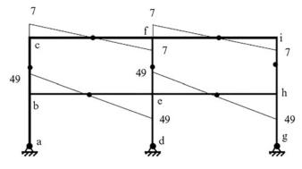
Fig. E11.1e Bending moment distribution for the beams (kN m)
