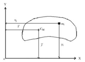
When the loading is dynamic, additional inertia forces are generated due to the acceleration of the masses located on the floor. In order to study the equilibrium of the floor, we need to establish the magnitude and location of the resultant of these inertia forces. In what follows, we describe the procedure for locating this resultant.
