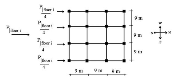
Fig. E15.2b Typical floor plan
