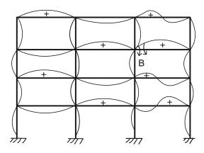
**Fig. 15.12** Deflection pattern for negative moment at B—inflection points in columns
