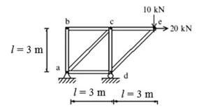
Fig. E2.14a Geometry and loading
