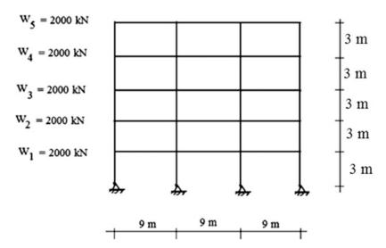
Fig. E14.16a Elevation
