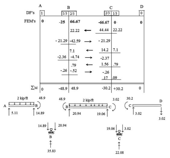
Fig. E10.12b Free body diagrams
