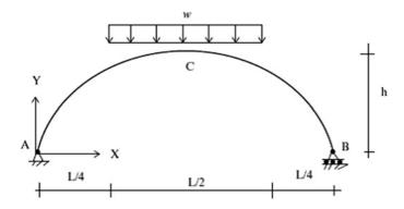
**Problem 6.9** Consider the parabolic member shown below. Determine the vertical displacement at C. Take  $I = 400 \text{ in.}^4$ ,  $A = 40 \text{ in.}^2$ ,  $E = 29,000 \text{ kip/in.}^2$
