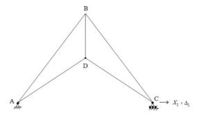
Fig. E9.16b Primary structure—redundant reaction
