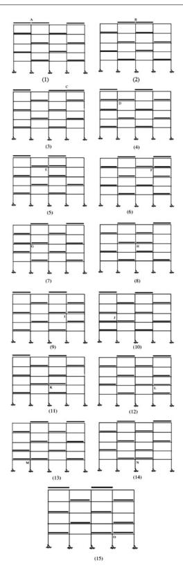
Fig. E15.1c Live load patterns for negative moment
