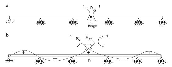
Fig. 13.4 Modified structure and deflected shape for positive moment at D
