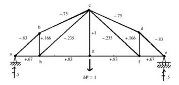
**Fig. E2.16c** Virtual forces,  $\delta F$  Using this data, the following computations are carried out:
