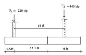
Fig. E7.4a Elevation
