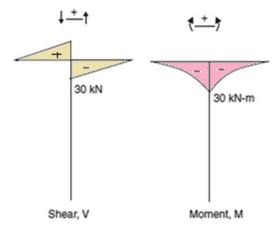
Fig. E4.2d Shear and moment diagrams
