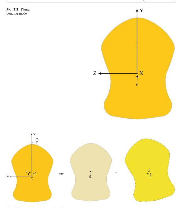
Fig. 3.4 Combined bending and torsion
