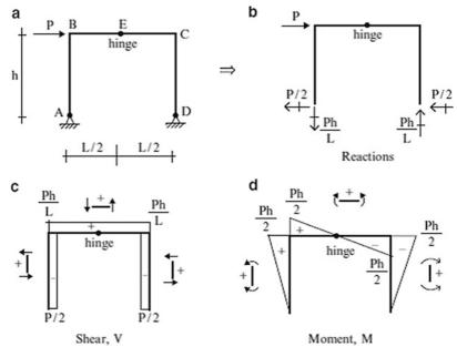
**Fig. 4.15** Variable cross-section 3-hinge frame
