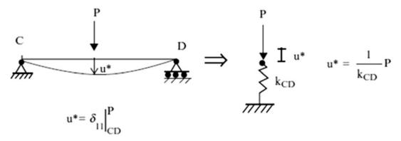
Fig. 9.20 Equivalent spring
