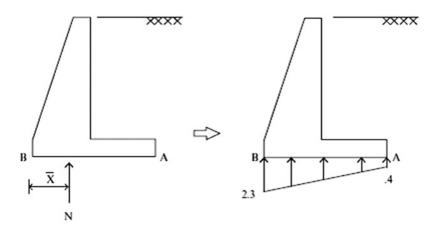
Case "B": For this case, we work with the free body diagram shown in Fig. E8.3e. The dimensions are defined in Fig. E8.3b.  $W_3 = (0.150)(6)(2)(1 \text{ ft}) = 1.8 \text{ kip}$ .  $W_5 = (0.120)(2)(2)(1 \text{ ft}) = 0.48 \text{ kip}$
