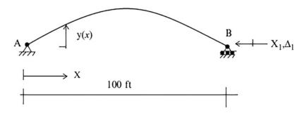
Fig. E9.13b Primary structure—redundant reaction
