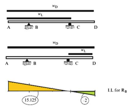
Fig. E3.25d Maximum and minimum values of  $R_{\rm B}$
