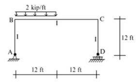
**Problem 4.35** Determine the displacement at the roller support C. Take E = 29,000 ksi and I = 100 in. Use the Virtual Force method.
