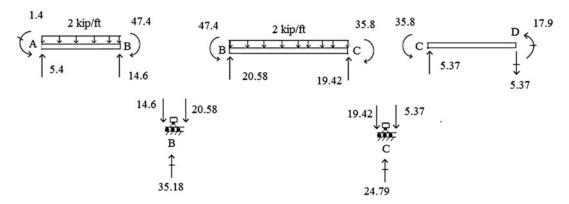
Fig. E10.11b Free body diagrams
