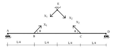
Fig. E9.5b Primary structure
