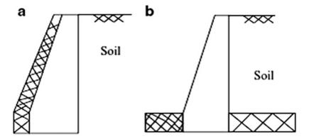
Fig. 8.13 (a) Gravity wall and (b) cantilever retaining wall
