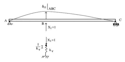
**Fig. E9.4b** Deflected shape due to  $X_1 = 1$
