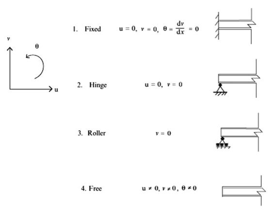
Fig. 3.25 Types of end conditions—displacement measures
