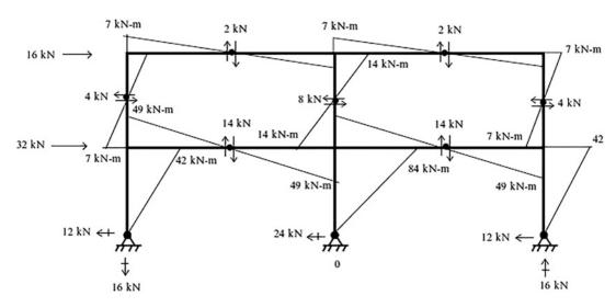
Fig. E11.1h Reactions, shear forces, and moment distribution
