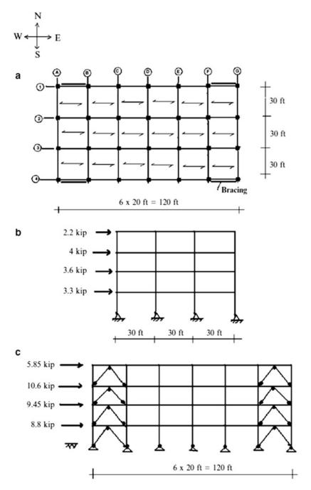
**Fig. 15.17** Rigid frame N–S, braced frame E–W. (a) Plan. (b)Typical rigid frame elevation—N–S; wind loading. (c) E–W elevation braced frames 1-1, 4-4; wind loading
