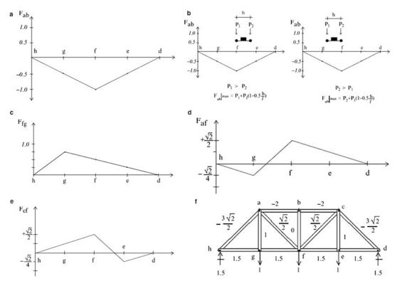
**Fig. 2.28** (a) Influence line for cord member ab. (b) Vehicle positioning for  $F_{ab}|_{max}$ . (c) Influence line for chord member fg. (d) Influence line for diagonal member af. (e) Influence line for diagonal member cf. (f) Uniform unit load
