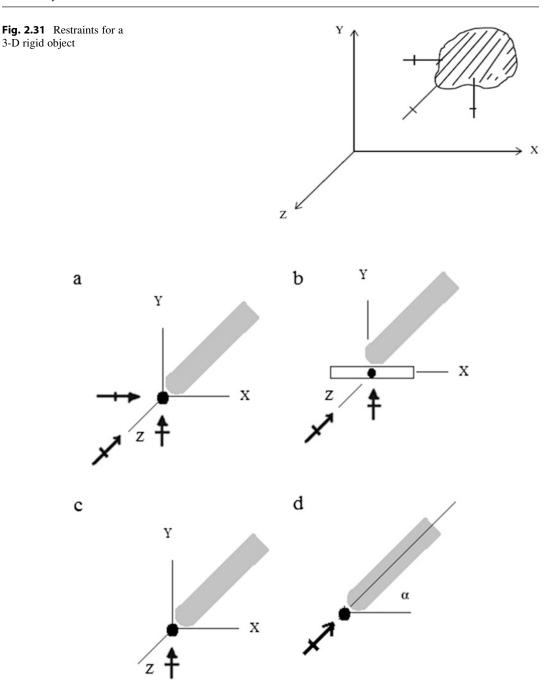
Fig. 2.32 Types of supports for space trusses. (a) Hinge joint. (b) Slotted roller. (c) Roller. (d) Rigid link
