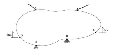
**Fig. 9.9** Displacement due to unit values of the redundant. (a)  $R_{\rm C}=1$ . (b)  $R_{\rm D}=1$
