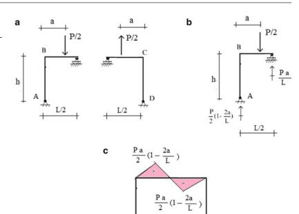
Fig. 9.42 Primary structure for two-hinged frame—symmetrical loading case
