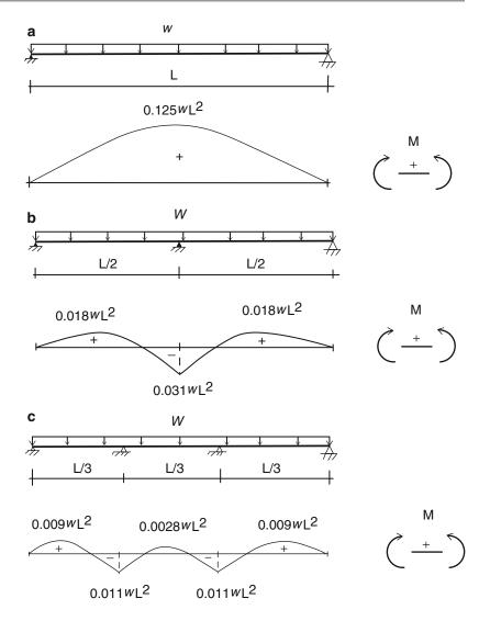
**Fig. 13.11** Bending moment distribution—three-span symmetrical scheme
