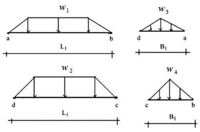
The floor loading is represented as a uniform load q (Ib/ft<sup>2</sup> or N/m<sup>2</sup>) applied to the floor slab. Using the concept of tributary areas, we convert this loading to a line loading w (Ib/ft or N/m) on the perimeter floor beams. The loading patterns for the beams supporting panel abcd and adjacent panels shown in Fig. 15.5 are listed below.
