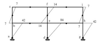
Fig. E11.1c Bending moment distribution for the columns  $(kN\ m)$
