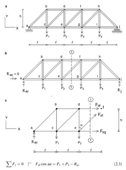
We point out here that the function of the diagonal members is to equilibrate the unbalanced vertical forces at the sections along the longitudinal axis. These forces are called "shear" forces.
