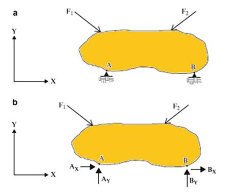
**Fig. 1.24** Definition of internal forces
