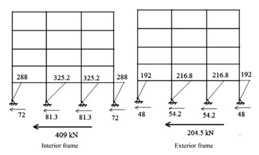
Fig. E14.16h Maximum column moments—flexible floors
