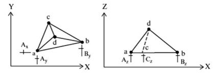
Fig. E2.21e Complete set of restraints
