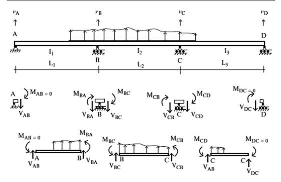
Fig. 10.12 Three-span beam
