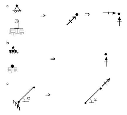
**Fig. 2.16** Types of supports for planar trusses. (a) Hinge support (two restraints  $\Rightarrow$  two reactions). (b) Roller Support (one restraint  $\Rightarrow$  one reaction). (c) Rigid link
