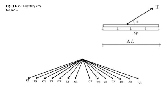
We estimate I for the girder by assuming the bending moment diagram is similar to the distribution for a uniformly loaded beam with multiple spans equal to  $\Delta L$ . The peak negative moment for this case is  $\frac{w(\Delta L)^2}{12}$ . Given these estimated properties, one analyzes the structure and iterates on the properties until the design requirements are satisfied.
