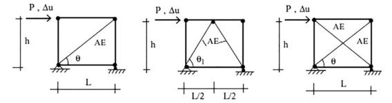
Fig. 11.16 Diagonal bracing systems. (a) Single. (b) Chevron. (c) X Brace
