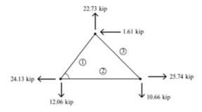
Fig. E12.9d Fixed end actions—joints
