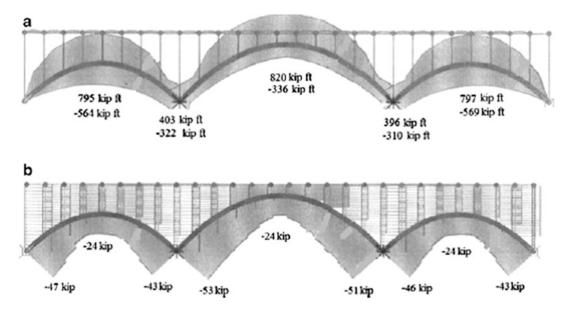
Fig. 13.32 Force envelopes—three-span arch. (a) Moment envelope—three-span arch. (b) Axial envelope—three-span arch
