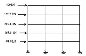
Fig. E14.16c Earthquake floor loads
