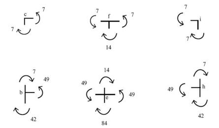
Fig. E11.1d Moments at the joints (kN m)
