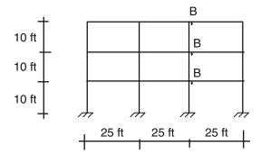
Using Müller-Breslau Principle, estimate the loading patterns (uniformly distributed member load) that produce the peak value of negative moment at B for each story. Check the results using a software package. Take  $I_c = 150$  in.<sup>4</sup> for all the columns and  $I_g = 300$  in.<sup>4</sup> for all the beams.
