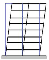
**Fig. 14.8** Lateral displacement profile with respect to ground
