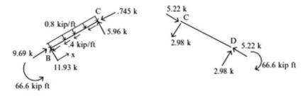
Fig. E4.10d End forces in local frame
