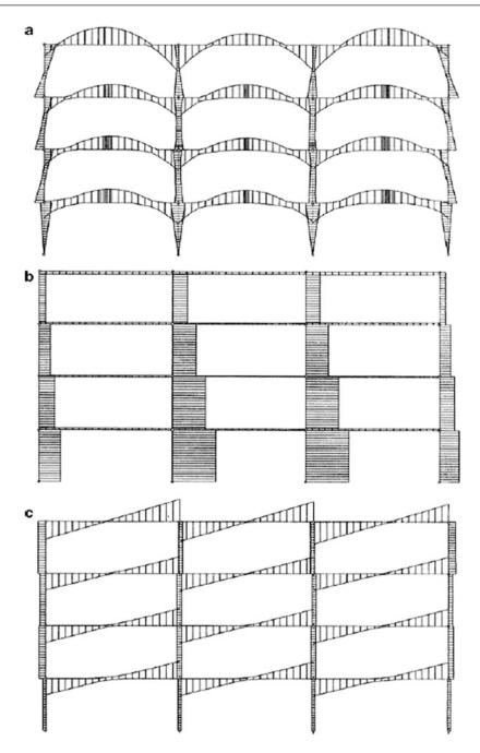
**Fig. 15.21** (a) Discrete moment envelope–factored load combination. (b) Discrete axial force envelope–factored load combination. (c) Discrete shear envelope–factored load combination
