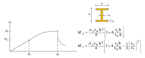
Fig. 16.5 Moment-curvature plot—thin walled wide flange section and EPPF material
