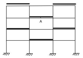
**Fig. 15.11** Deflection pattern for negative moment at B—inflection points in beams
