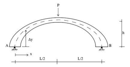
Fig. E9.12a Variable depth arch
