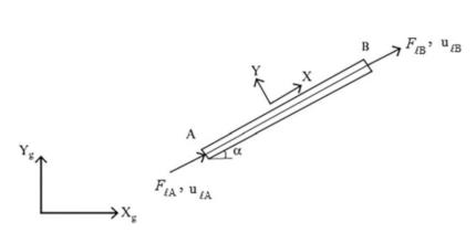
Fig. 12.7 End force and end displacement—local member truss—planar behavior
