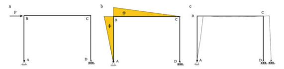
Fig. 4.31 Portal frame. (a) Loading. (b) Bending moment. (c) Deflection profile
