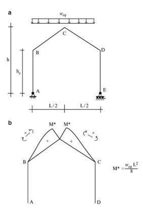
**Fig. 4.21** 3-Hinge frame under gravity loading. (a) Structure and loading. (b) Moment diagram
