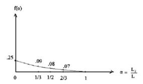
Taking  $L_2 = L_1$  corresponds to  $\alpha = 1/3$ . The more common case is where  $\alpha$  is between 1/3 and 1/2. When spans  $L_1$  and  $L_2$  are chosen, one applies the uniformly distributed loading and determines the peak value of negative moment using (13.5).
