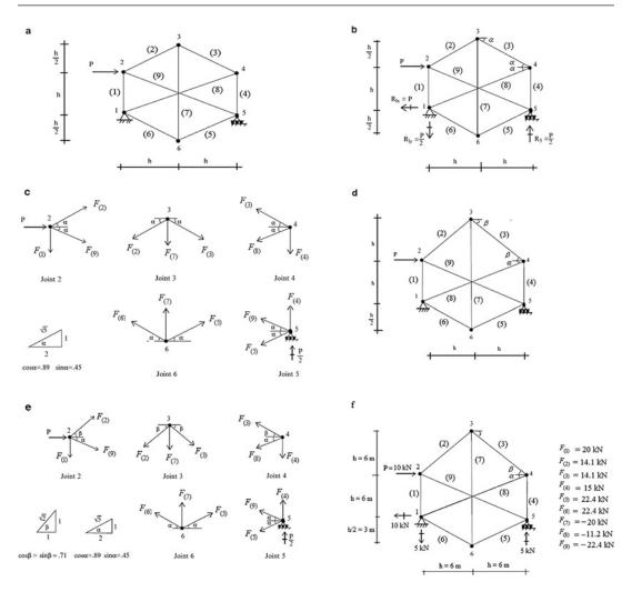
Fig. 2.20 (a) Planar truss geometry. (b) Reactions. (c) Joint equilibrium. (d) Modified geometry. (e) Joint equilibrium. (f) Member forces
