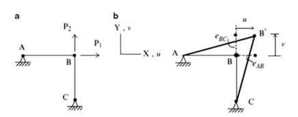
**Fig. 2.23** Extension displacement relationships
