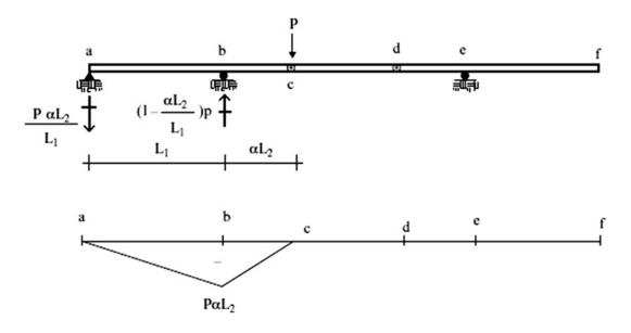
Fig. E3.27c Moment diagram—load on member BC
