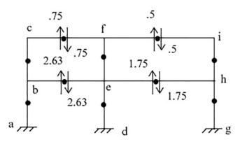
Fig. E11.2f Shear distribution for the beams (kip)
