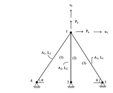
**Fig. 10.3** Extension and force quantities—axial loaded member
