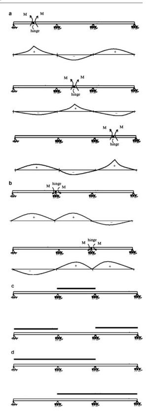
Given the loading patterns, one generates the bending moment distribution for each loading condition and then establishes the maximum values of the positive and negative moments at the *same discrete locations* selected for the truck loading. These results define the discrete moment envelope for the structure. Four separate analyses (cases 1–4) are required to construct the discrete moment envelope corresponding to the lane loading for this three-span example.
