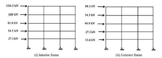
Fig. E14.16f Frame loads—flexible floors
