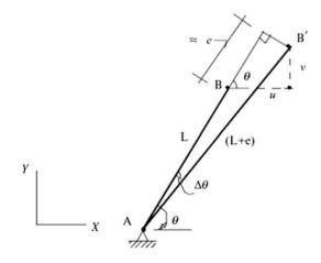
**Fig. 2.24** Geometry—two-member truss
