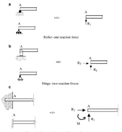
Clamped-three reactions (two forces and one moment)
