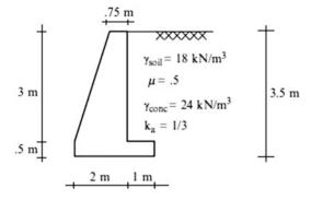
**Problem 8.3** For the concrete retaining wall shown, determine the factors of safety against sliding and overturning and the base pressure distribution. Use the Rankine theory for soil pressure computations
