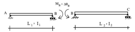
Fig. E9.10b Primary structure—redundant moment
