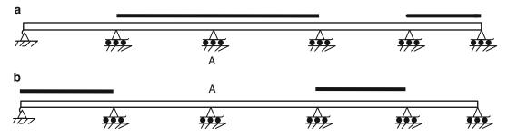
Fig. 13.3 Loading zones for moment at A. (a) Negative moment at A. (b) Positive moment at A
