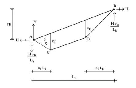
Example 5.2 Analysis of an Inclined Cable
