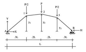
**Problem 6.18** Determine the optimal shape of the arch for a given value of H. Assume L = 30 m and  $w_0 = 15$  kN/m.
