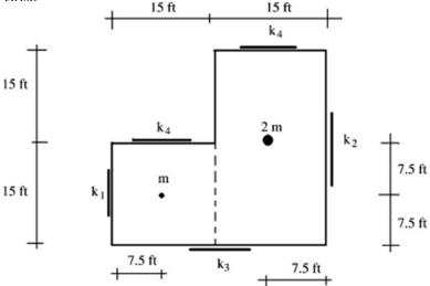
**Problem 14.10** Consider the floor plan shown below. Assume the mass is uniformly distributed over the floor area. Establish the equations of motion referred to point O.
