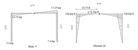
Fig. E4.5g Shear and moment diagrams
