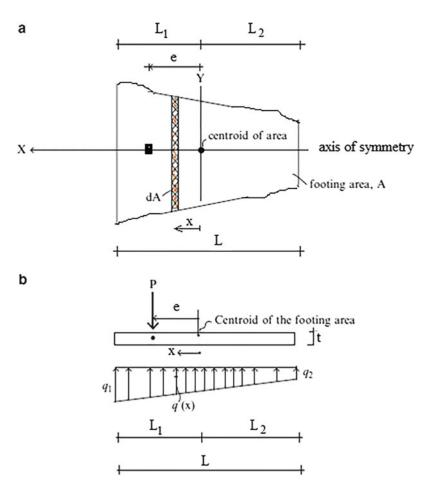
Fig. 7.7 Notation-pressure distribution-single footing. (a) Plan. (b) Elevation
