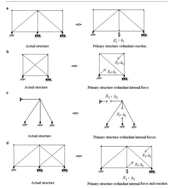
Fig. 9.56 Examples of statically indeterminate trusses
