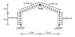
For the A-frames defined in Problems 4.27–4.29, determine the reactions and bending moment distribution.
