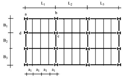
**Fig. 15.7** One-way action beam loading for uniform floor loading q. (a) Large joist spacing. (b) Small joist spacing
