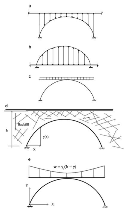
**Fig. 6.11** Different roadway arrangements—idealized loading. (a) Roadway above the arch. (b) Roadway below the arch. (c) Idealized uniform dead loading. (d) Soil backfill above the arch. (e) Idealized soil loading
