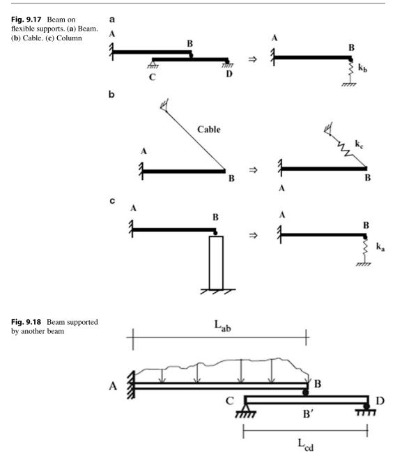
behave as linear elastic restraints, and can be modeled as equivalent spring elements, as indicated in Fig. 9.17.
