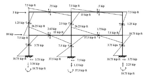
Fig. E11.2h Reactions, shear forces and moment distribution
