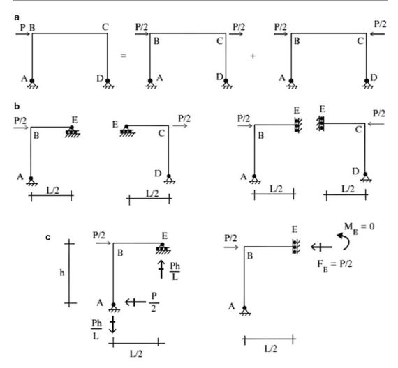
Fig. 9.38 Structural models. (a) Decomposition into anti-symmetrical and symmetrical loadings. (b) Anti-symmetric and symmetrical models. (c) Free body diagrams of anti-symmetric and symmetrical segments
