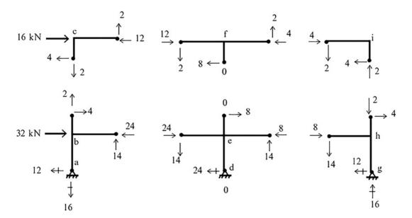
Fig. E11.1g Axial and shear forces (kN)
