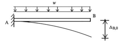
Fig. E9.1c Displacement due to external loading
