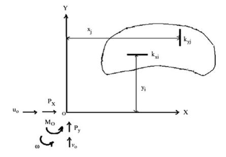
identify the various braces. Each brace is characterized by a stiffness magnitude (k) and the perpendicular distance from the tangent to the origin.
