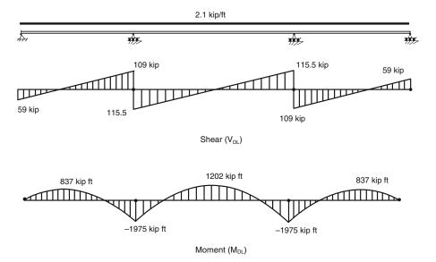
Fig. 13.23 Dead load shear and moment distributions
