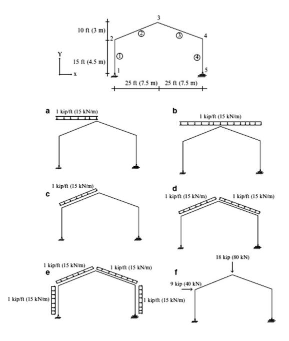
**Problem 4.42** Consider the frame shown below. Determine the required minimum *I* for the frame to limit the horizontal deflection at C to 0.5 in. The material is steel. Use computer software.
