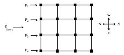
Fig. E14.16d Floor load distribution
