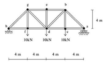
Fig. E2.6a Bridge truss
