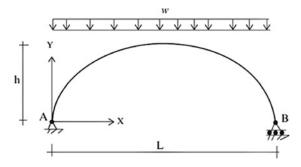
Fig. E6.1a Parabolic geometry
