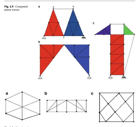
Fig. 2.5 Complex planar trusses
