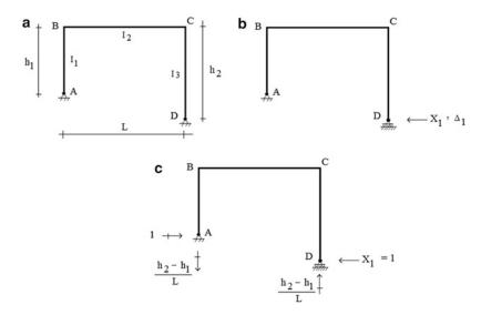
**Fig. 9.34** Reactions—gravity loading
