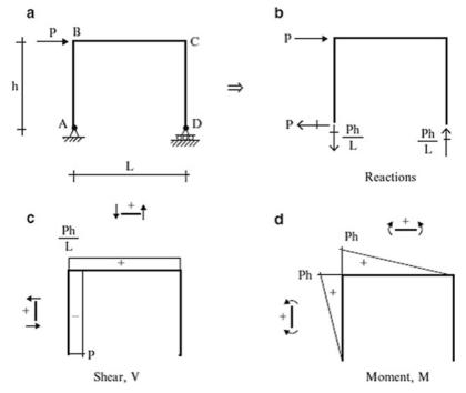
Fig. 4.13 Statically determinate 3-hinge portal frame under gravity loading. (a) Geometry and loading. (b) Reactions. (c) Shear diagram. (d) Moment diagram
