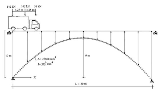
Fig. 13.28 Parabolic-arch geometry and loading-idealized model
