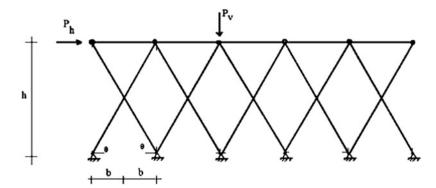
**Problem 15.11** For the structure shown below, assume the floors are flexible and the flooring system transits the gravity loading to the floor beams in the N–S direction (one-way action). Assume all beams are the same size and all the columns are the same size.  $I_{\text{beam}} = 3I_{\text{column}}$ , Floor<sub>gravity</sub> = 175 kN/m<sup>2</sup>.
