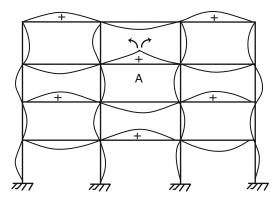
**Fig. 15.10** Loading pattern for maximum positive moment at A
