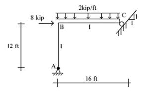
**Problem 4.36** Determine the horizontal deflection at C and the rotation at joint B. Take E = 200 GPa and  $I = 60(10)^6$  mm<sup>4</sup>. Use the Virtual Force method.
