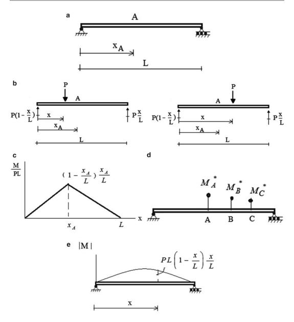
**Fig. 3.50** (a) Beam. (b) Loading patterns – Concentrated load P at  $x < x_A$  and  $x > x_A$ . (c) Moment diagram. (d) Different load patterns. (e) Moment diagram. (f) Shear diagrams for concentrated load P at  $x < x_A$  and  $x > x_A$ . (g) Influence line for shear at location  $x_A$ . (h) Maximum and minimum shear. (i) Shear force envelope
