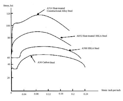
measure is the rupture strain  $\varepsilon_r$ . By definition,  $\varepsilon_r$  is the fractional change in length of the specimen and is usually expressed as a percentage. For mild steel, the percent elongation is about 24 %. Ductility refers to the ability to deform plastically without fracturing and is measured by the ratio  $\frac{\varepsilon_r}{\varepsilon_v}$ . This ratio
