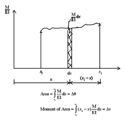
**Fig. 3.27** Graphic interpolation of (3.26)
