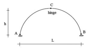
Problem 6.12 Consider the semicircular three-hinged arch shown below. Determine the vertical and horizontal displacements at C due to the loading.
