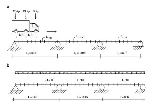
Fig. 13.22 Span discretization for live loads. (a) Truck. (b) Lane load
