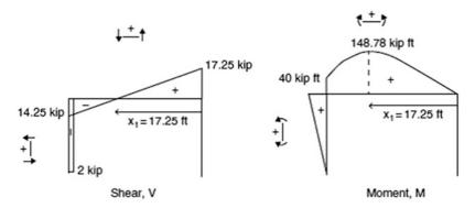
Fig. E4.4d Shear and moment diagrams
