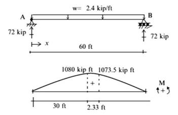
**Fig. E3.30d** Moment distribution for dead load When there are multiple loadings, it is more convenient to generate discrete moment envelope using a computer-based analysis system. The discrete moment envelope for the combined (dead + truck) loading is plotted below (Fig. E3.30e). Scanning the envelope shows that the maximum moment occurs at x = 30.9 ft and  $M_{\text{max}} = 1882.6$  kip ft. This result shows that it was reasonable to superimpose the moment diagrams in this example.
