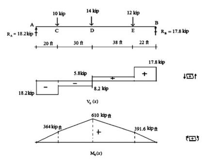
Fig. E5.1b Simply supported beam results
