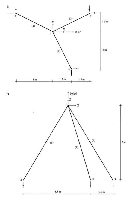
Fig. E12.13 Space truss geometry and supports. (a) x-y plan view. (b) x-z plan view
