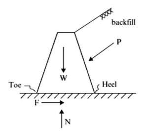
Fig. 8.2 Free body diagram—gravity structure
