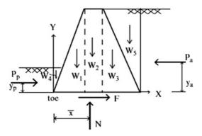
Fig. 8.12 Typical gravity wall
