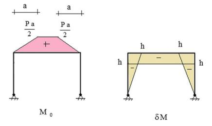
**Fig. 9.44** Final bending moment distribution
