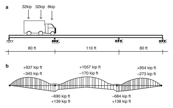
Fig. 13.33 Force envelopes—three-span girder. (a) Geometry and loading. (b) Moment envelope
