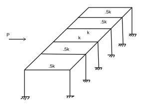
**Problem 14.6** Consider the stiffness distribution for the one-story rigid frame shown below. Determine the displaced configuration under the action of the loading shown. Assume the slab is rigid.
