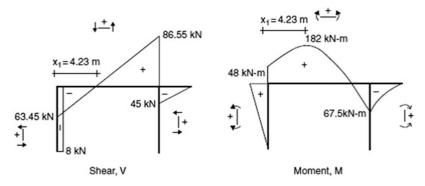
Fig. E4.6d Shear and moment diagrams
