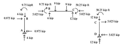
Fig. E10.8d Free body diagrams
