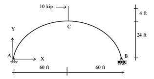
**Problem 6.4** Determine the reactions, the axial and shear forces, and the moments at x = 30 ft for the three-hinged parabolic arch shown below.
