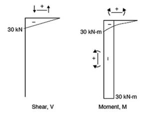
Fig. E4.1d Shear and moment diagrams
