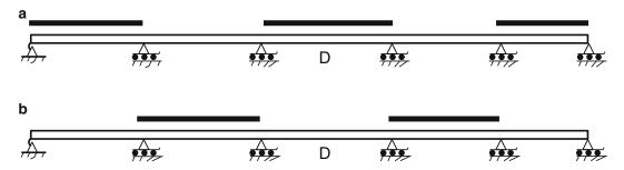
Fig. 13.5 Loading zones for moment at D. (a) Positive value. (b) Negative value
