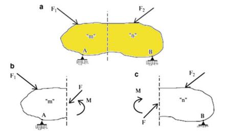
reactions which are "external forces." Note that the magnitude of the internal forces varies with the location of the cutting plane. The following example illustrates the process of computing internal forces.
