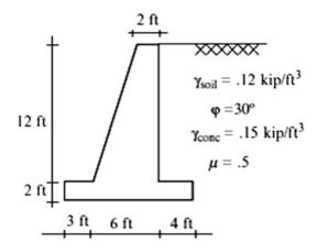
**Problem 8.4** For the concrete retaining wall shown, determine the required value for  $b_2$ . Take the factors of safety for overturning and sliding to be equal to 1.75 and 1.25, respectively. Use the Rankine theory for soil pressure computations.
