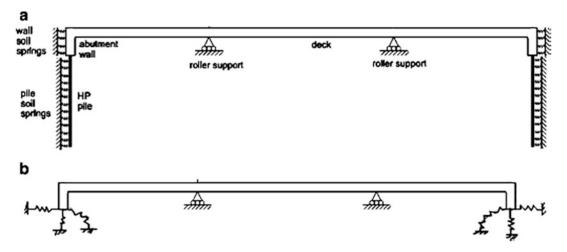
Fig. 13.9 Idealized models for an integral abutment bridge (a) Global model. (b) Simplified model
