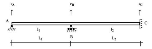
Fig. 10.11 Beam geometry and support settlements
