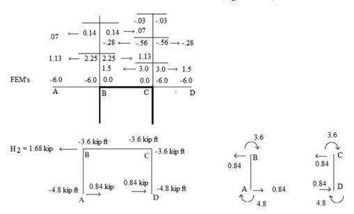
Fig. E10.17e Case II—end moments and column shear
