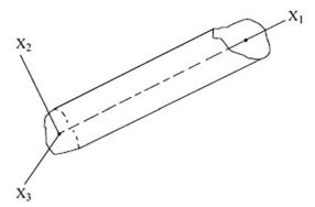
**Fig. 12.10** End displacements and forces in local coordinate system
