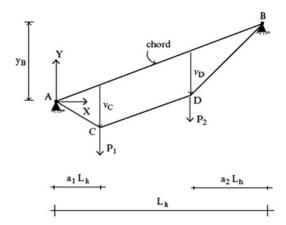
When the cable is inclined, we follow the same approach except that now we measure the *cable sag* with respect to the inclined chord. Consider the cable defined in Fig. 5.10. This example differs from the previous examples only with respect to the inclination of the chord AB.
