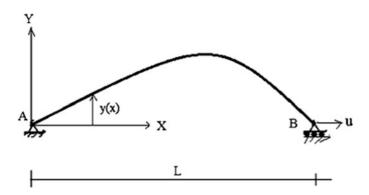
**Problem 6.8** Consider the parabolic member shown below. Determine the horizontal displacement at B.
