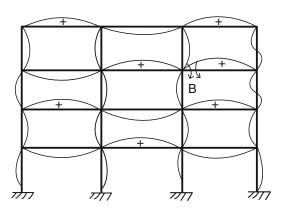
or the beams. These shapes are plotted in Figs. 15.11 and 15.12. The exact shape depends on the relative stiffness of the beams and columns which is not known at the preliminary design phase. Although there are cases where there is some ambiguity in the deflected shape, the Müller-Breslau Principle is a very useful tool for generating a qualitative first estimate of the loading pattern (Fig. 15.13). One can refine the estimate later using a structural analysis software system.
