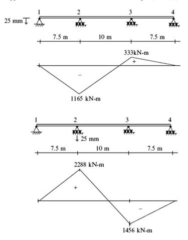
**Fig. E13.2b** Case a results Case a: L = 10 m
