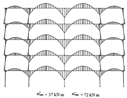
Fig. E15.1e Moment diagram for uniform loading
