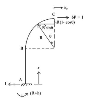
**Fig. E6.4d**  $\delta M(x)$  for  $u_c$
