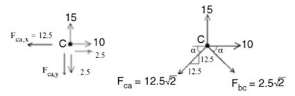
Fig. E2.4d Joint C
