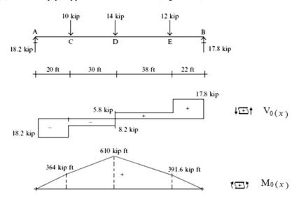
Fig. E5.2b Simply supported beam results
