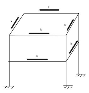
**Problem 14.5** Consider the single-story multi-frame structure shown below. Determine the lateral forcef in the frames due to a global load P. Consider both wind and earthquake loading. Assume the slab is rigid.
