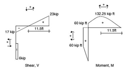
Fig. E4.3d Shear and moment diagrams
