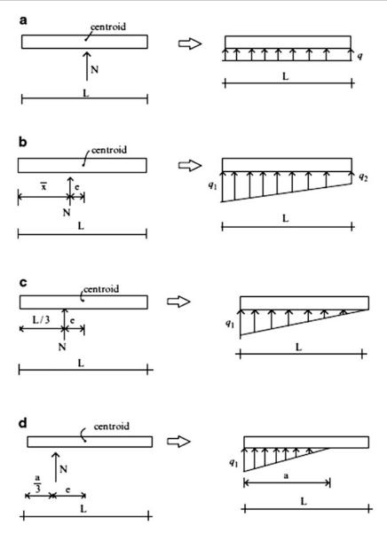
**Fig. 8.14** Pressure distributions on footing/wall base. (a) e = 0. (b) e < L/6. (c) e = L/6. (d) e > L/6
