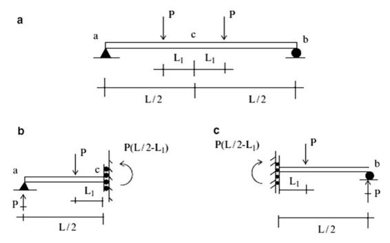
Fig. 3.48 Boundary conditions on symmetry axis—symmetrical planar loading. (a) Symmetrical load. (b) Left segment. (c) Right segment
