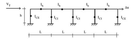
**Fig. 11.12** Typical :sub-elements for base story—fixed support. (a) Exterior. (b) Interior
