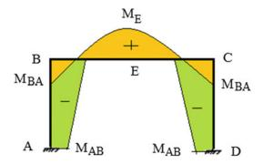
Fig. 9.50 Bending moment distribution symmetrical loading hinged supports
