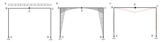
Fig. 4.28 3-Hinge frame. (a) Loading. (b) Bending moment. (c) Deflection profile
