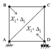
Fig. E9.17b Primary structure—internal force redundant
