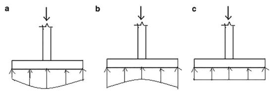
Fig. 7.5 Soil pressure distributions—concentric load. (a) Sandy soil. (b) Clayey soil. (c) Average soil pressure
