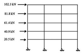
Fig. E14.16e Frame load—rigid floors
