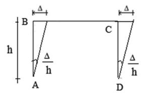
Fig. E10.17d Case II—sideway introduced
