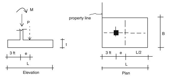
Fig. E7.2b Geometry and loading
