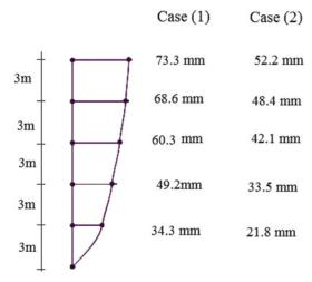
Fig. E15.2g Lateral displacement of the floors—earthquake
