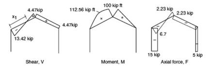
Fig. E4.9e Internal force diagrams
