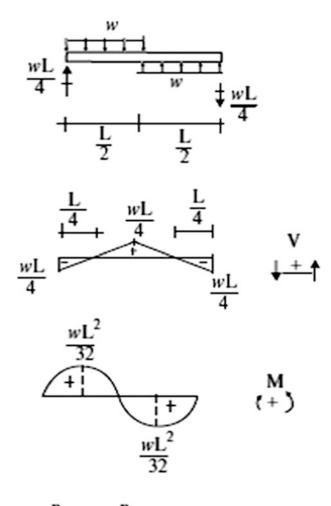
**Fig. 3.42** Antisymmetrical 2-point loading
