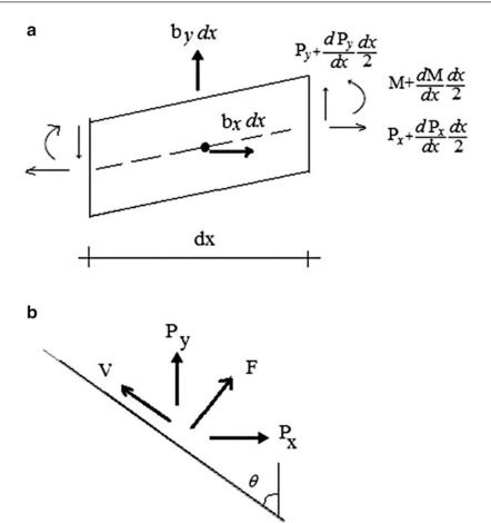
Fig. 10.33 (a) Differential element (b) Cartesian components
