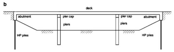
Fig. 13.8 (a) Three-span integral abutment bridge in Orange, Massachusetts. (b) Elevation—three-span integral abutment bridge
