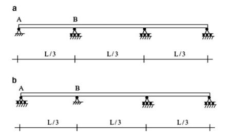
**Problem 13.5** Most design codes limit the deflection due to live loading to some fraction of length, say  $L/\alpha$ , where  $\alpha$  is on the order of 500. Generate the global "deflection" envelope for the multi-span beam and truck loading shown below. Take E=29,000 ksi and I=60,000 in.<sup>4</sup>
