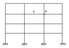
**Fig. 15.9** Deflection pattern for positive moment at A
