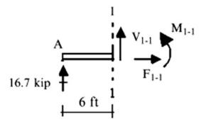
Fig. E1.3c Left segment-cutting plane 1-1
