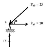
$$\sum F_y = 0 \quad F_{ab,y} = 15 \downarrow \quad \therefore F_{ab} = 25 \, \text{kip (compression)}$$
