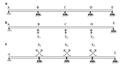
Fig. 9.14 (a) Actual structure. (b) Primary structure—redundant reactions. (c) Primary structure—redundant internal forces
