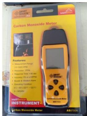
Gambar 3.21. Gas *Detector AS8700A*
