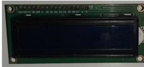
Gambar 3.16. *Blue LCD 16x2 Display*
