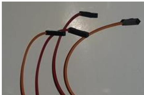
Gambar 3.8. *Female Jumper Wire*
