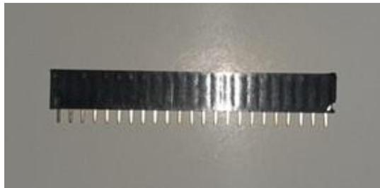
Gambar 3.9. *Straight Female Header Pin*
