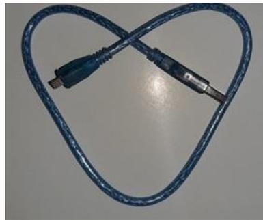
Gambar 3.11. *Micro USB to B Cable*
